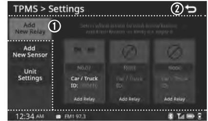
① Add New Relay control screen: Shows current wheel layout, Vehicle ID, and Add Relay button of each vehicle type
