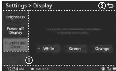
❶ **Illumination Colour** controls: Sets colour of the illumination (tab) about Faceplate buttons light.
