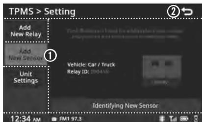
① Add New Sensor control screen: Shows current vehicle type, Relay ID and wheel layout.
